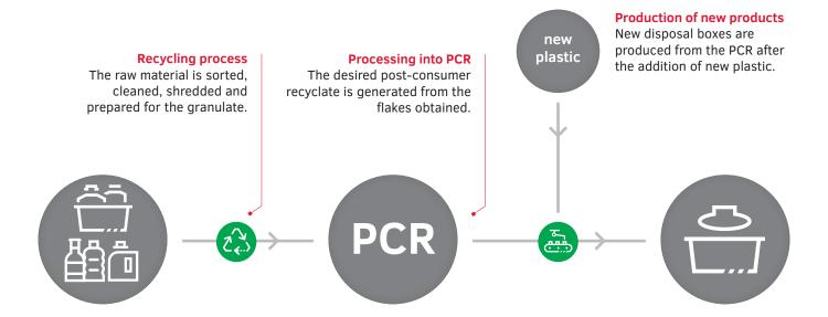
Used plastic packaging, such as yogurt pots, is turned into so-called **post-consumer recyclate (PCR)**. Together with **new plastic** -- to ensure the highest quality standards - this recycled material is used in the production of new waste disposal boxes, with a recycled content of up to 61%\*. Resource-saving and sustainable.
